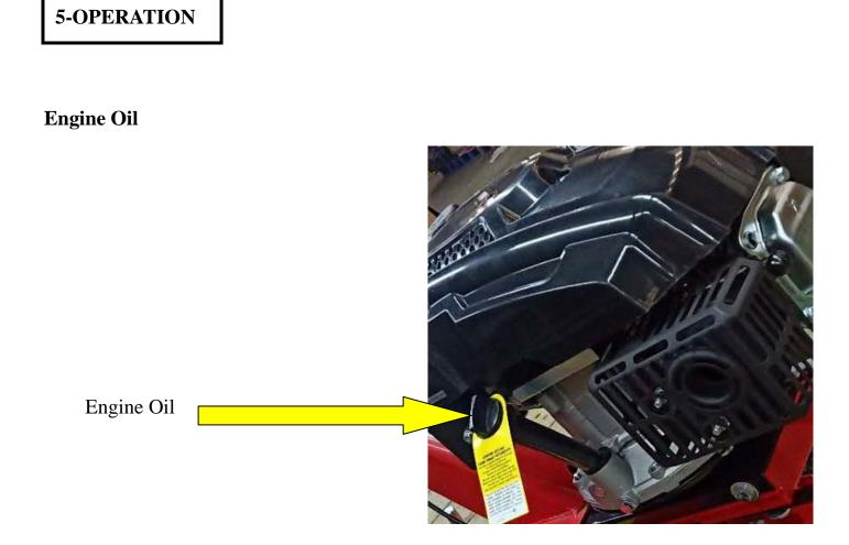
**Warning:** Engine delivered without oil, please add 0.50 liter of oil before use. Oil should be changed for the first time after 2 hours, then replace engine oil every 30 hours. Inspect oil lever before each time use. The oil lever must always be between the MAX and the MIN sign on dipstick.
