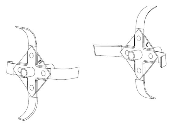
Note: L means left blade, which is different from right blade(R). L and R are engraved on the blade.
